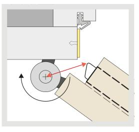
$\textcircled$  high drop height, large floor gap  $\Theta$  small drop height, small floor gap
