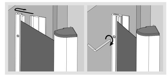
The easy clip-on system developed by Planet allows you to effortlessly install the textile profile and then tighten it up easily with the Allen key. (FSR 6000 / FSR 7000)
