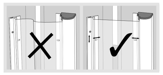
The position of both the finger protection blind and the suspension profile can be moved to the left and right, and the textile profile can be moved up and down if required. (FSR 6000 / FSR 7000)
